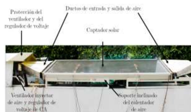
Figure 2 View of the solar air heater
