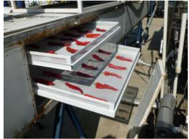
Figure 3 Disposal of fresh chili peppers in the drying chamber
