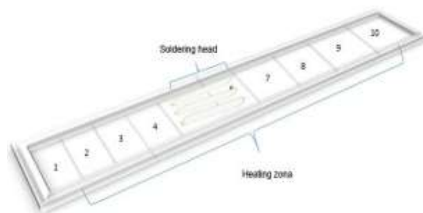
Figure 7 Scheme of preheating zones (1, 2, 3, 4) and of welding (5, 6) of Stringer Machine Own Elaboration
