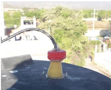
Figure 6 Installation of the Ultrasonic Sensor in Tinaco Own Elaboration
