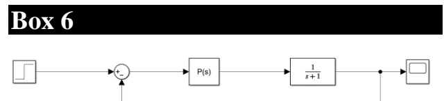
Figure 6 Control system for performing transfer function tuning
