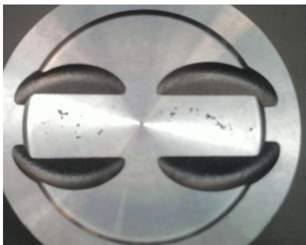
Figure 2 Pore in the head of a piston
