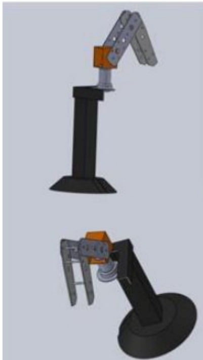
Figure 1 CAD design of robot type PUMA BY 3GDL
