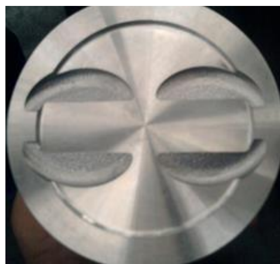
Figure 12 Piston free of imperfections
