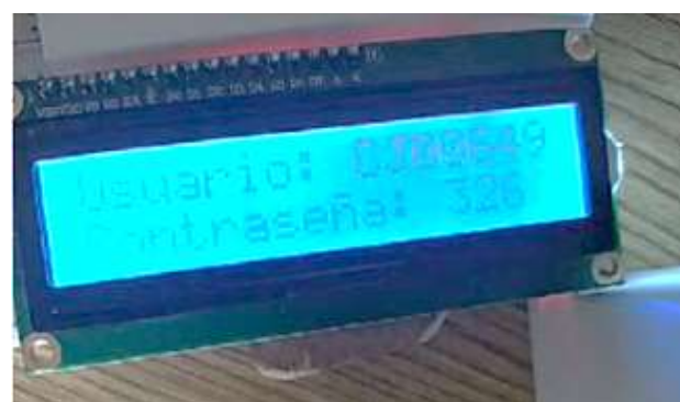
Figure 10 LCD screen showing the user and Password that has been acquired.
