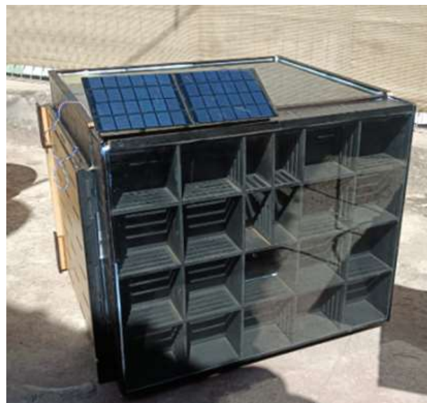
Figure 10 Final finish of the solar dryer Source: Own elaboration
