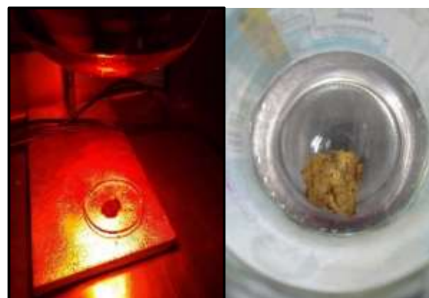
Figure 2 Paraphidippus aurantius spider silk drying in infrared light
