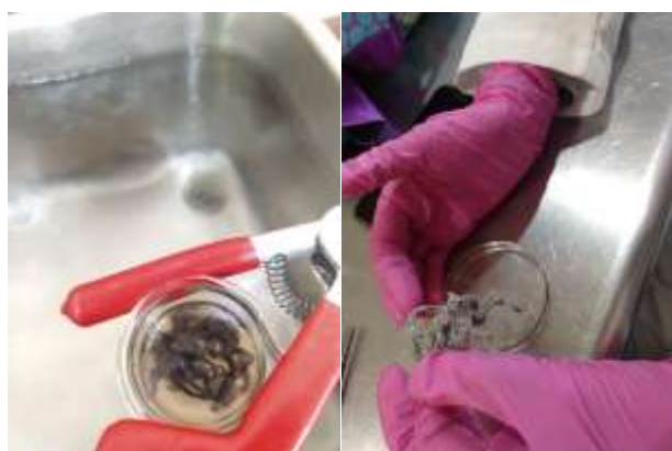
Figure 3 Spider silk cleaning and sonication process
