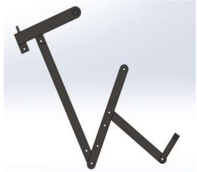
Figure 4 SolidWorks design for the six-bar Watt linkage mechanism is presented. It is important to notice that the smallest link at the right corresponds to the motor connection. The link on the left generates the leg movement. The holes in the middle links allow reconfiguring to have a smaller range of motion.
