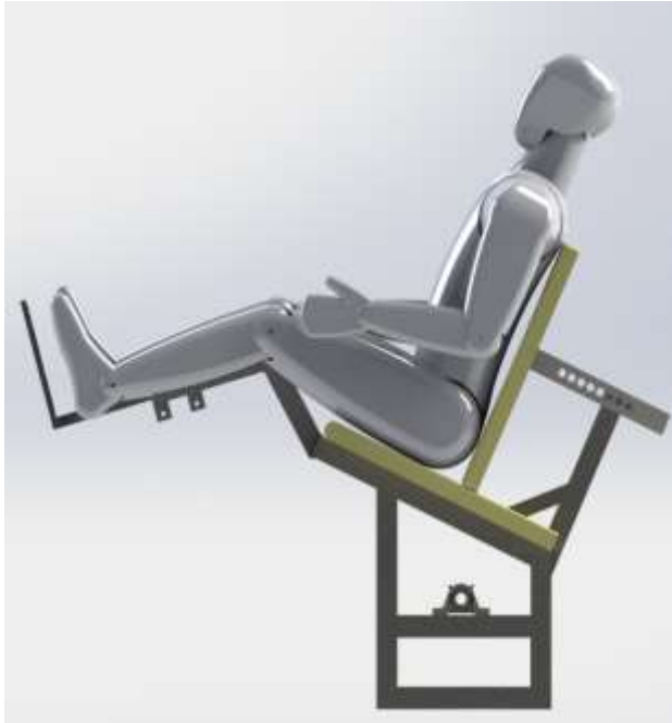
Figure 2 SolidWorks model of the original extension machine where is possible to see that it depends on the person to generate the movement.
