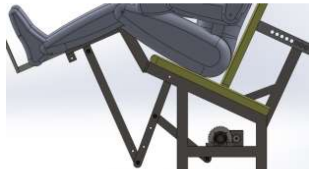
Figure 6 The assembly is presented with the six-bar Watt linkage placed into the machine. Notice that a rowlock is the support for the transmission gear, while the motor is fixed with an iron base
