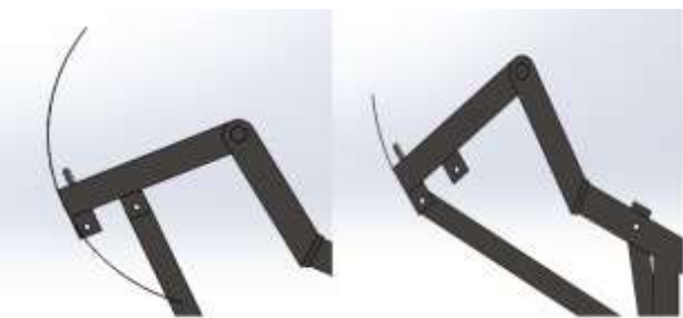
Figure 8 Trace path of the configurations with the widest ( a – 109.28°) and shortest ( h – 24.23°) range of motion, respectively. Notice the variation in the last link from left, it causes to have a greater effort in the case a .
