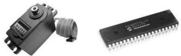
Figura 1 Servomotor MG995 y microcontrolador PIC 16F877A
