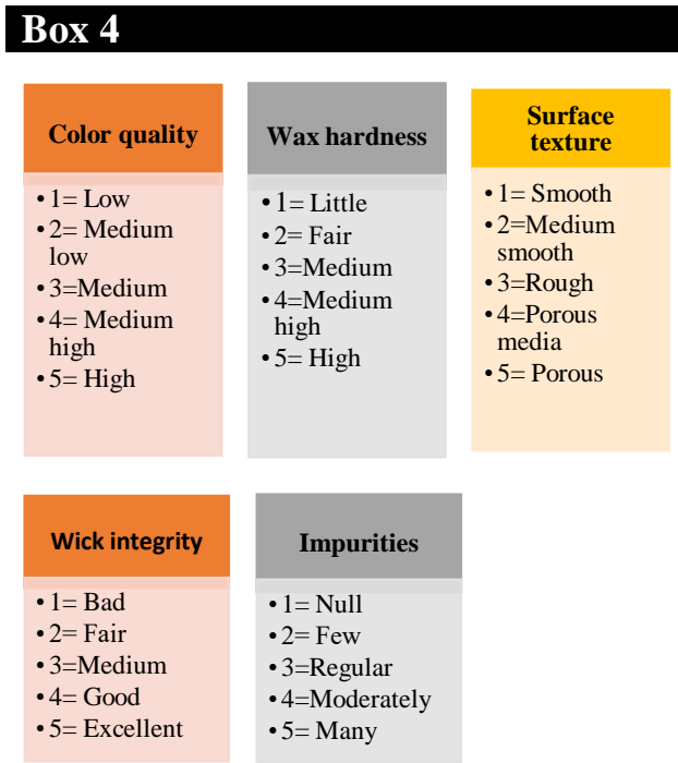
Figure 4 Value scale for the Visual and Physical Inspections test Own elaboration
