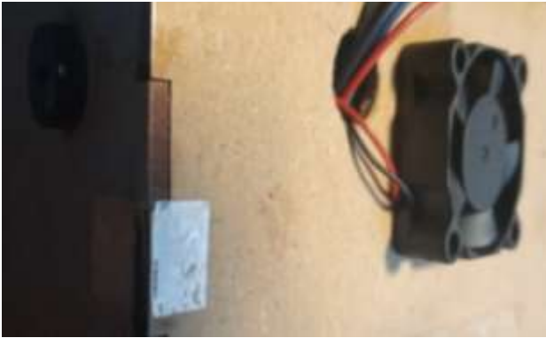
Figure 4 Rear of gas detector device, buzzer and fan Source: Own Elaboration
