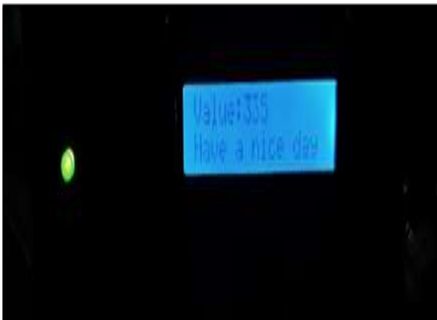
Figure 5 Actuators of the device when no gas is detected in the environment Source: Own Elaboration
