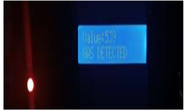
Figure 6 Actuators of the device when gas is detected in the environment Source: Own Elaboration
