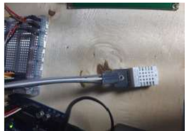
Figure 4 Use of temperature and humidity sensor
