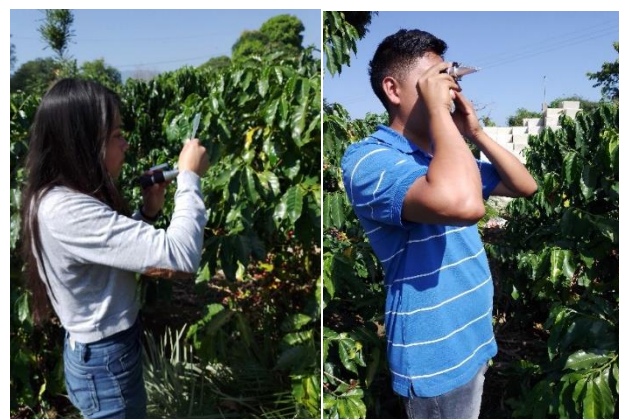
Figure 3 Sample of the Brix measurement with the refractometer at Rancho Las Palmas and Rancho Doña Juana
