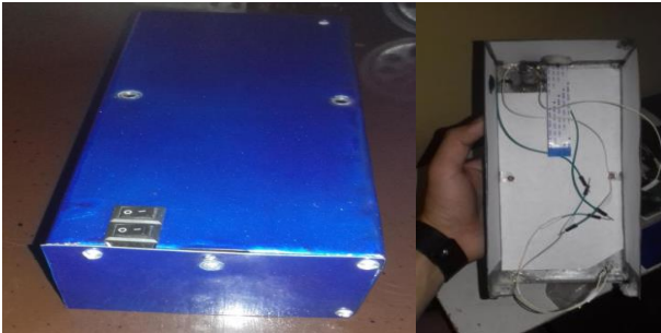
Figure 6 Circuit protective shell. The left Figure shows the exterior of the protective case and its power button. The Figure to the right shows the inside of the protective case and the connections of the power button with the Raspberry Pi
