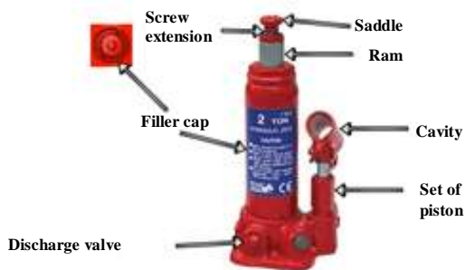
Figure 2 Parts of a bottle-type hydraulic jack
