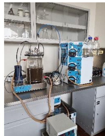
Figure 1 Photo-Sequential Bach Reactor (SBR) used in experimental biogranulation process
