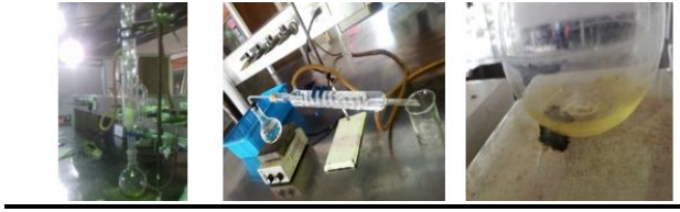
Figure 5 Fats and oils extraction, soxhlet method, Figure 6 Hexane recovery, Figure 7 Extracted hydrocarbons
