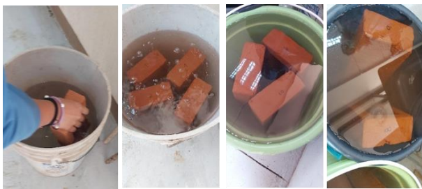
Figure 5 Bricks immersed in water for absorption test. Source: Own elaboration
