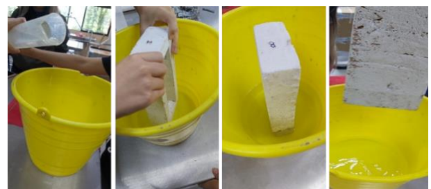
Figure Absorption test process with waterproofing Source: Own elaboration
