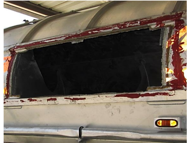
Figure 2 The image shows the original fracture of the vessel and the fracture of the weld joining the patch. Evidence of the polymer placed on the edge of the patch plate (red spot) was found Source: own work [Canon powershot A3400IS]
