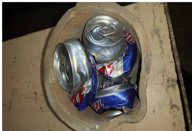
**Figure 2** Clay pot for casting
