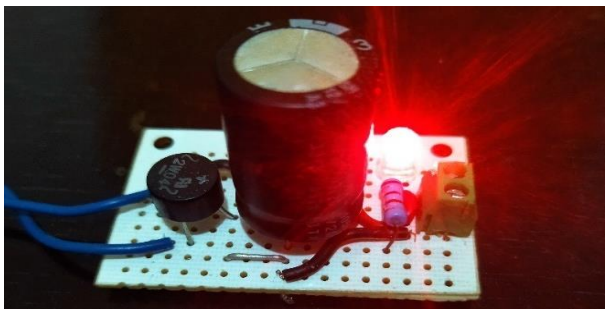
Figure 16 Test of the source, and the indicator led Source: own elaboration
