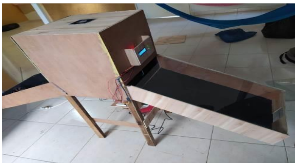
Figure 24 Assembly of the LCD display, and the indicator LEDs Source: own elaboration
