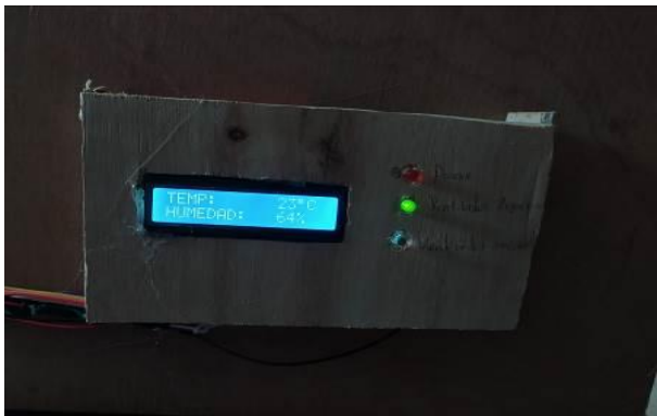
Figure 23 Assembly of the LCD display, and the indicator LEDs Source: own design
