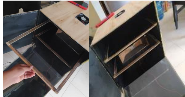
Figure 21 Assembly of the collectors to the drying cabinet, and the installation of the nets Source: own elaboration
