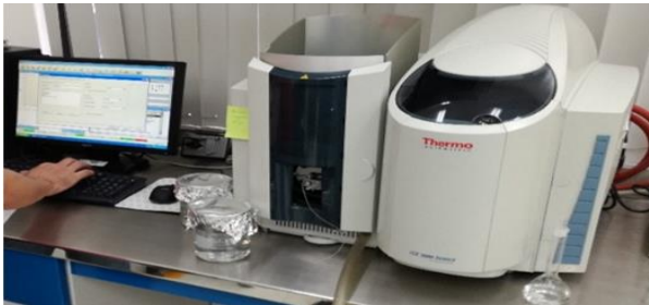
Figure 6 Atomic absorption equipment Source: CIAD 2017
