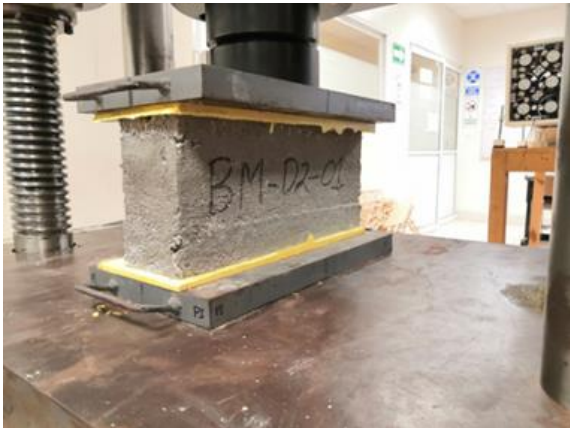
Figure 3 Laying of blocks for compression testing
