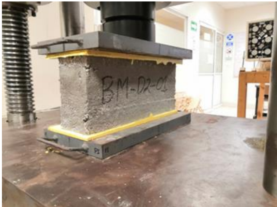
Figure 3 Laying of blocks for compression testing
