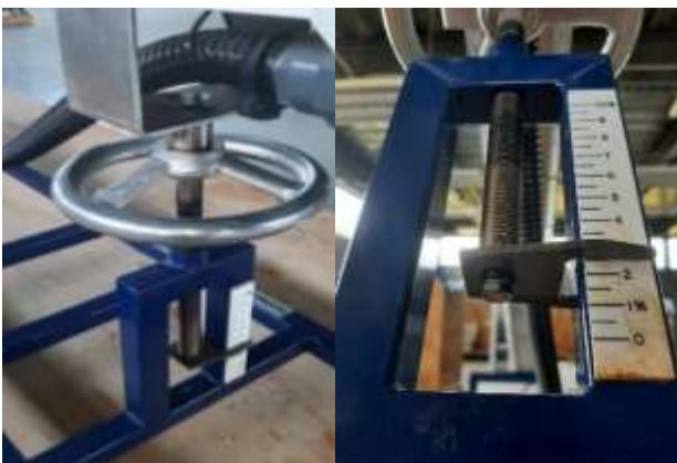
Figure 3 Manual mechanism for slope adjustment
