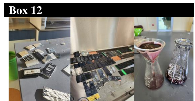
Figure 12 Disassembly, leaching, and filtering of battery cathodes.
