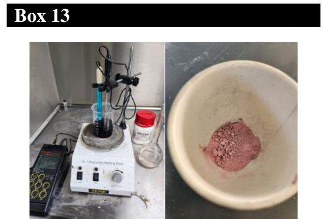
Figure 13 Addition of ammonium oxalate and precipitation of cobalt oxalate.
