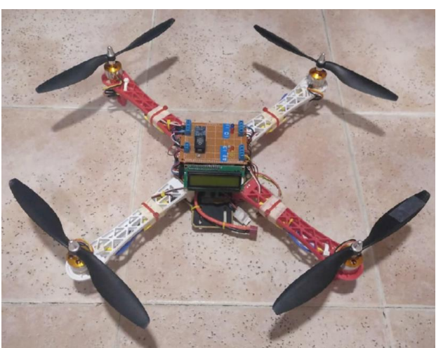
Figure 5 Drone based on Arduino and open source technologies Source: [Gómez, 2020]
