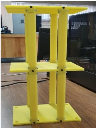
Figure 1 Academic test rig printed in 3D
