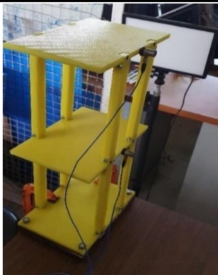
Figure 3 Placement of Accelerometers
