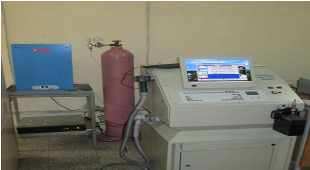
Figure 2 Optical emission spectral analysis equipment Source: Spectrographer's Handbook, 2015
