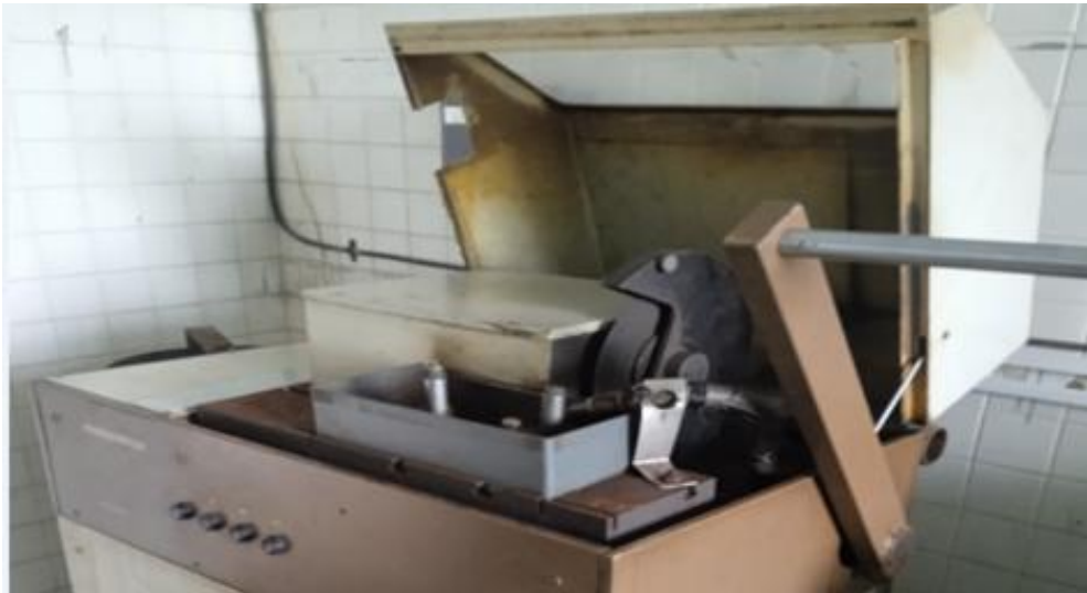
Figure 3 Metal cutting machine with abrasive disc Source: Own elaboration
