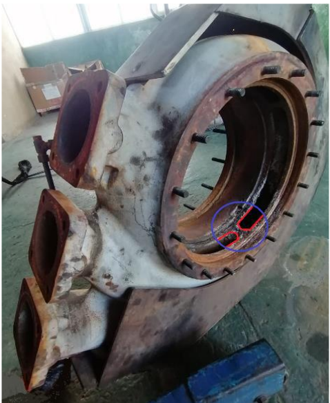
Figure 1 Turbine casing belonging to a turbocharger of the Generator Sets
