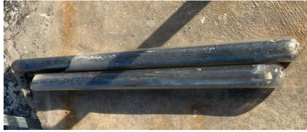
Figure 2 Failed evacuated tube
