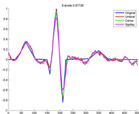
Figure 4 Filter a synthetic signal, using the process in Figure 2, with wn = DB34 , L = 6 and K = 4 .
