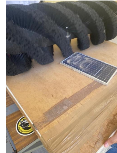
Fig. 8 Cleaning applied to photovoltaic modules with dry cleaning prototype.
