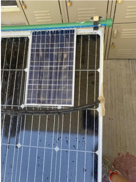
Fig. 7 Cleaning applied to photovoltaic modules with wet cleaning prototype.
