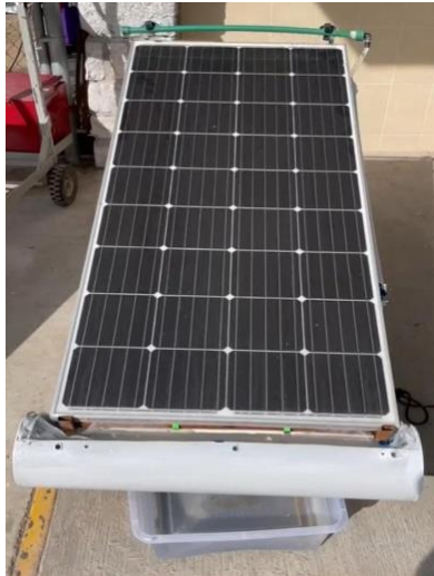
Fig. 5 Wet cleaning prototype [Own source]
