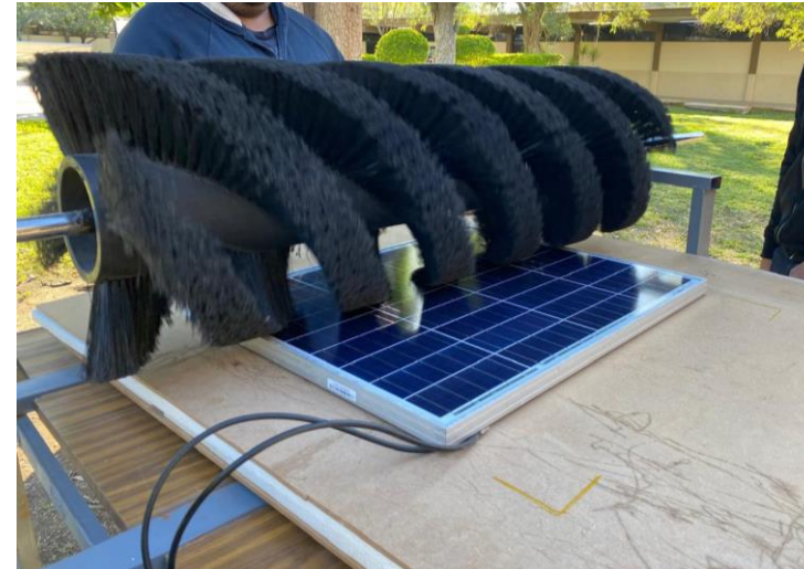
Fig. 6 Dry cleaning prototype [Own source]
