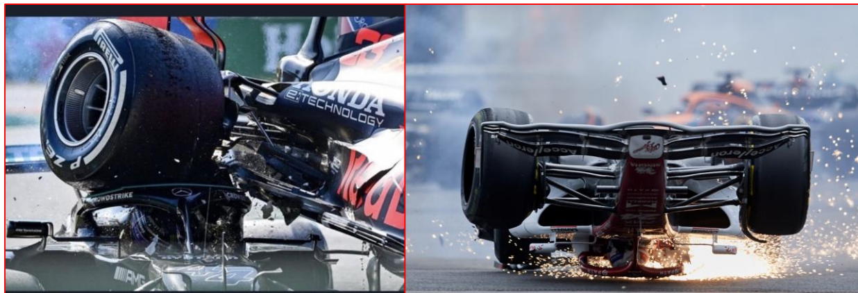
Figure 2. Halo device protection against objects and rollovers
