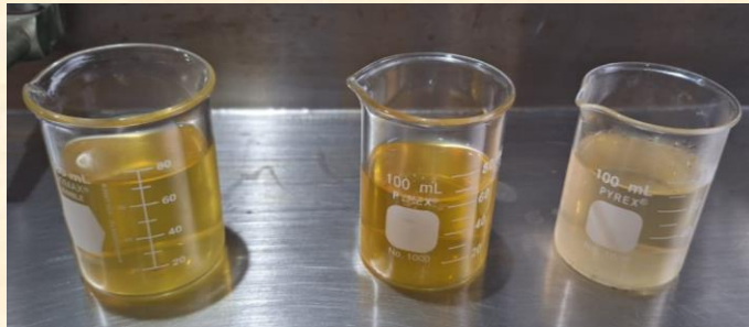
Figure 1. Homogeneous solutions with piloncillo as a precursor and base of NH 3 (right vessel), NaOH (medium vessel) and HCl (left vessel)
