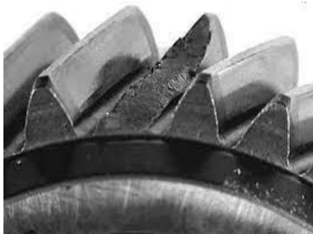
Figure 2. Gear with fractured tooth.
