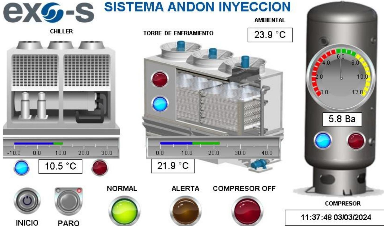
The final design of the ANDON system visualization, operating and running online, is shown in Figure. This graphic can be accessed by any internet-connected device for remote monitoring and operation. Access to this graphic is available from any point in the production plant via screens that display graphs and numerical indicators showing real-time values of process variables.
