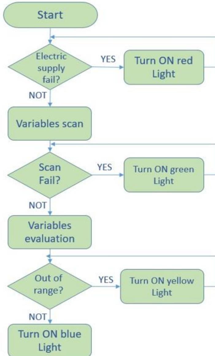
Considering the needs of the plant, it is required to monitor a failure in the electrical supply. Measure the values of temperature and pressure variables in real time, identifying that they remain within the desired range for production.
