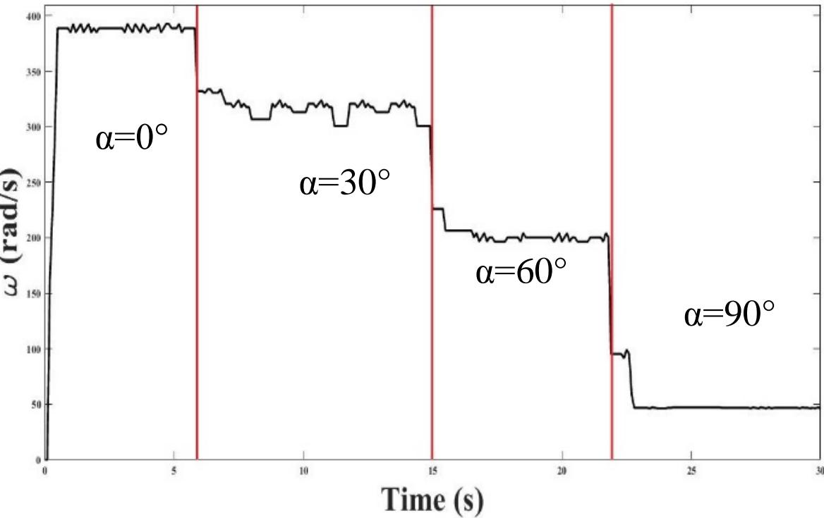
The relationship between the input and output variable corresponds to the firing angle ( $\alpha$ ) and the angular velocity ( $\omega$ ).
