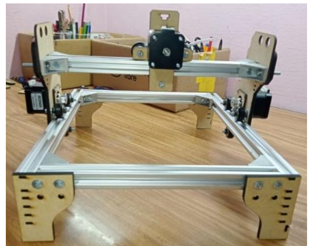
Figure 5 Prototype laser engraver with 2 axes and main structure
