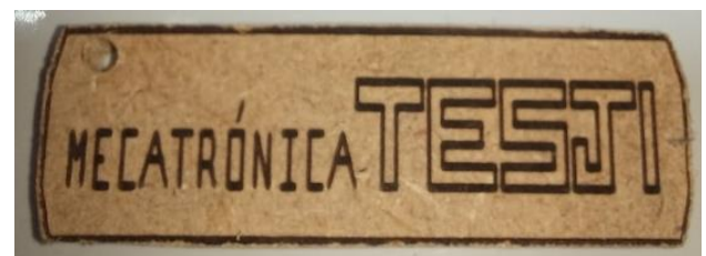
Figure 9 Etching test on MDF Source (project contribution, unpublished)
