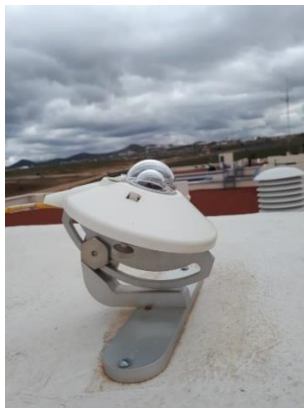
Figure 8 Global radiation pyranometer on inclined plane
