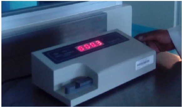
Figure 4 Measurement of hardness of rosemary extract tablets (Laboratory of Pharmacy, Chemical Sciences, UAZ, 2016).
