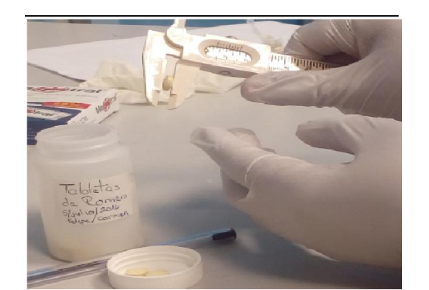
Figure 3 Measurement of the thickness of rosemary extract tablets (Pharmacy Laboratory, Chemical Sciences, UAZ, 2016) Own elaboration
