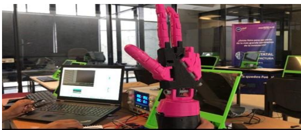
Figure 3 Detection of manual gestures and translation into prosthetic movements
