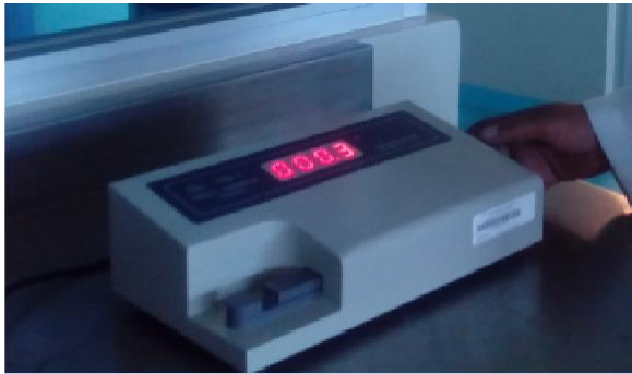
Figure 4 Measurement of hardness of rosemary extract tablets (Laboratory of Pharmacy, Chemical Sciences, UAZ, 2016).
