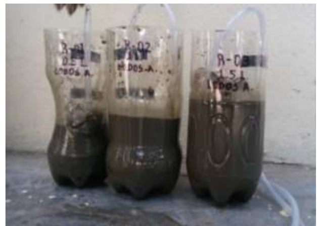
Figure 2 Termite isoptera reactors with sample of disposable nappies in place Source: Project collaboration team, 2020
