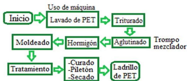
Figure 2 Process flow diagram for the production of environmentally friendly PET bricks
