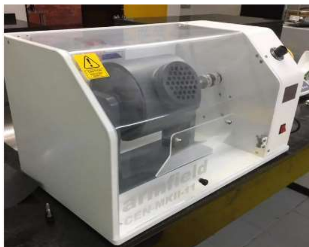
Figure 7 Armfield CEN-MKII-11 didactic ball mill Source: Own Elaboration
