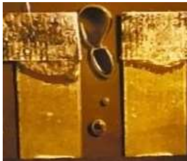
Figure 1 Plugs after Damp Heat Test
