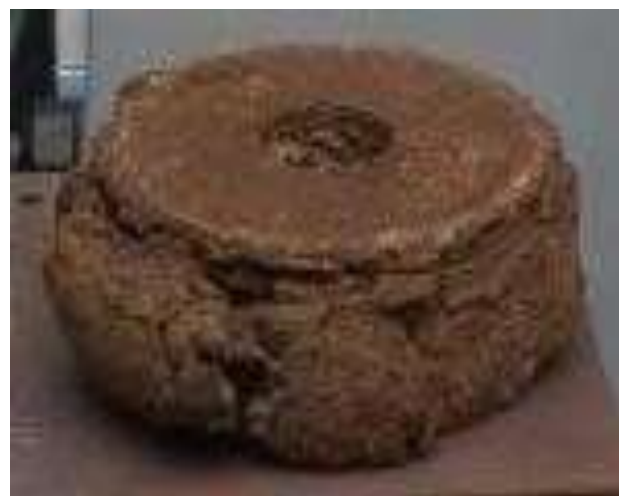
Figure 8 Final appearance of briquette after compression test Source: Own Elaboration
